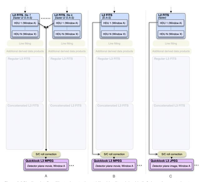
Figure 3-5 Pipeline dataflow (illustration starting at L2): wide-slit and dumbbell. Column A: repeated raster or repeated sit-and-stare. Column B: single sit-and-stare. Column C: single raster
