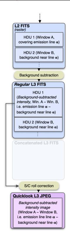
Figure 3-4: Intensity-window, single raster. The spectral binning factor is equal to the window width. It is also possible to create a stand-alone intensity-window without an associated background (or line) window. In such cases no background subtraction is performed, and the L3 R and L2 data arrays will be identical.
