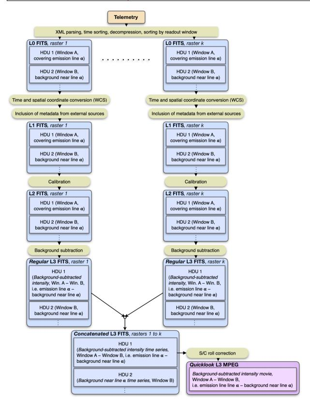
Figure 3-3: Intensity-window, repeated rasters. The spectral binning factor is equal to the window width. It is also possible to create a stand-alone intensity-window without an associated background (or line) window. In such cases no background subtraction is performed, and the L3 R and L2 data arrays will be identical.
